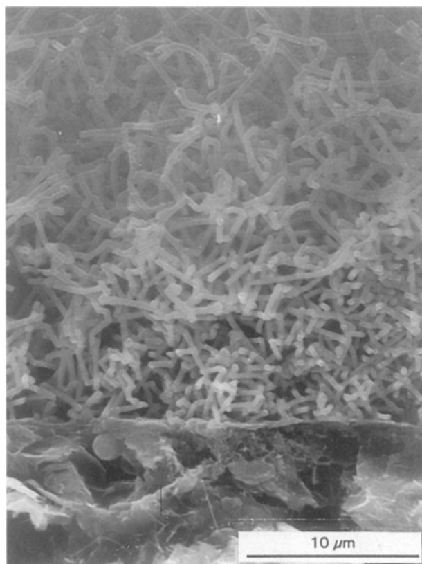
Figure 2 Cross-sectional view of SiC whisker mat on graphite substrate.
